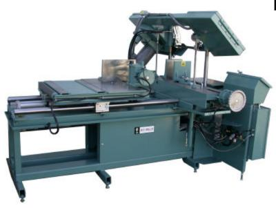
The W-914-A CNC utilizes a digital membrane touch screen to access all of the standard machine controls. The screen has been specially designed for use in a shop environment. To make it easier for the operator, the keys have a light to show which are active. The two-line display prompts the operator with easy-to-read, 3/8" high letters.
